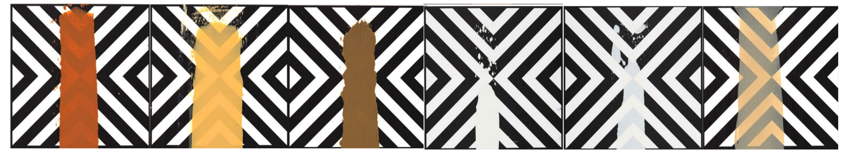
Fig. 12: A few of the oil-bound grounds tested in this study applied on opacity chart (red ochre, yellow ochre, raw umber, lead white and clay). The ground composed of lead white is applied in two different thicknesses.
